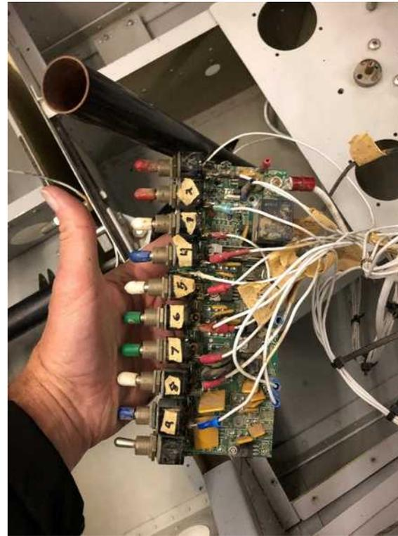
EXP-II voltage load center - replaced with standard circuit breakers and switches
