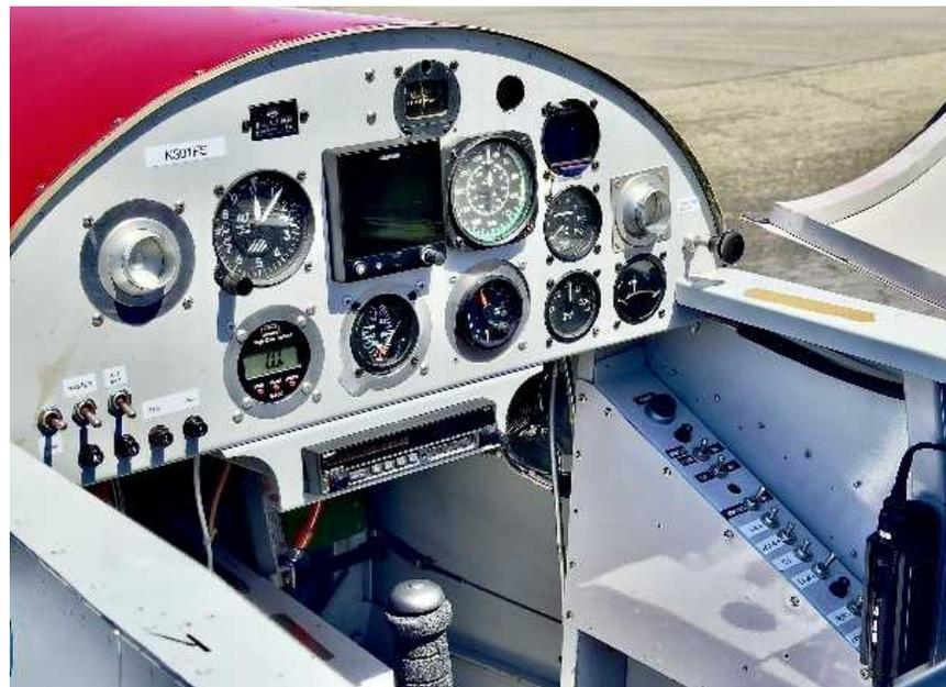
Vacuum system removed and replaced with a Garmin G5
