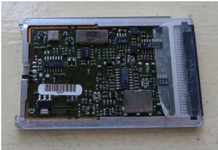
Early 802.11 radio card by Symbol Technologies – radio and microcomputer, 1 MBPS FH
