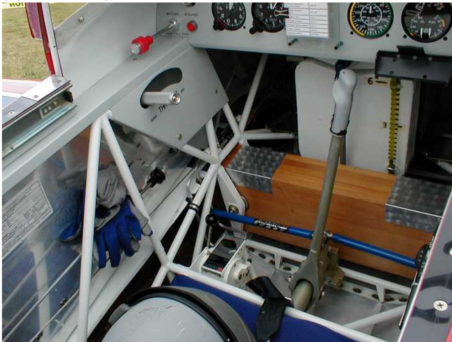
DR-107 Spar and Stick with support tube structure
