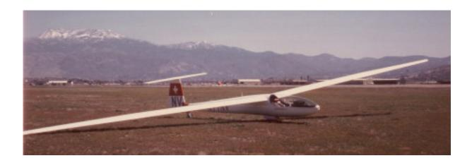
The Diamant: Manufacturer is "Flug- und Fahrzeugwerke Altenrhein" in Switzerland, commonly abbreviated FFA; the model is Diamant 18 (for its 18m/59 foot wingspan). The Diamant is fiberglass and has a 45:1 glide ratio.
