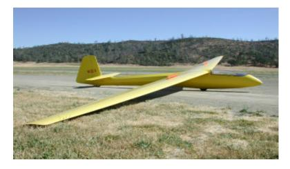
The Zugvogel: Manufacturer is Scheibe; Zugvogel IIIB (roman 3) is the model designation. Wingspan is 17m / 56 feet. The Zugvogel has wood wings and tail, tube and rag fuselage, and glides around 35 or 36:1.
